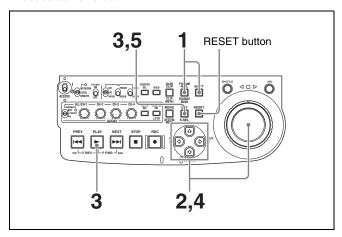
1 Hold down the SHIFT button, and press the THUMBNAIL button, turning it on.
